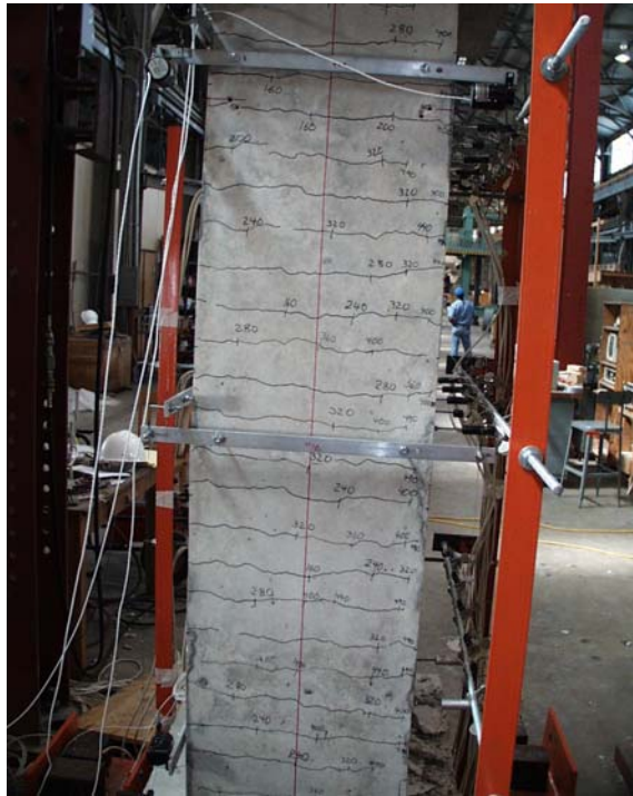
Figure 5.48 Specimen P12: Photo of South Wall at End of Test
