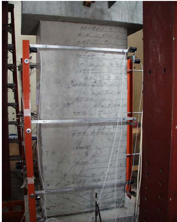
Figure 5.46 Specimen P12: Photo of West Wall at End of Test
