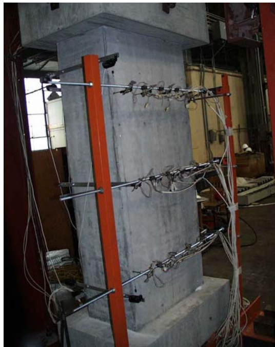
Figure 4.29 Linear Potentiometers to Measure Wall Profile Before Test
