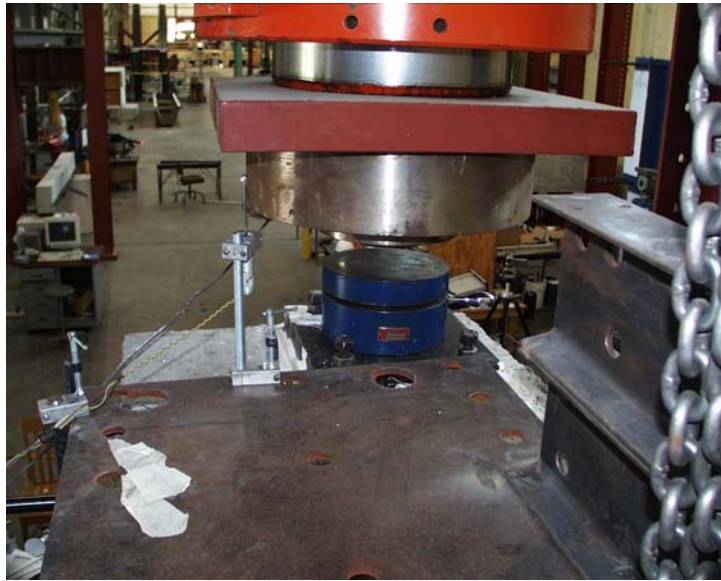
Figure 4.27 Spherical Bearing at Top End Block
