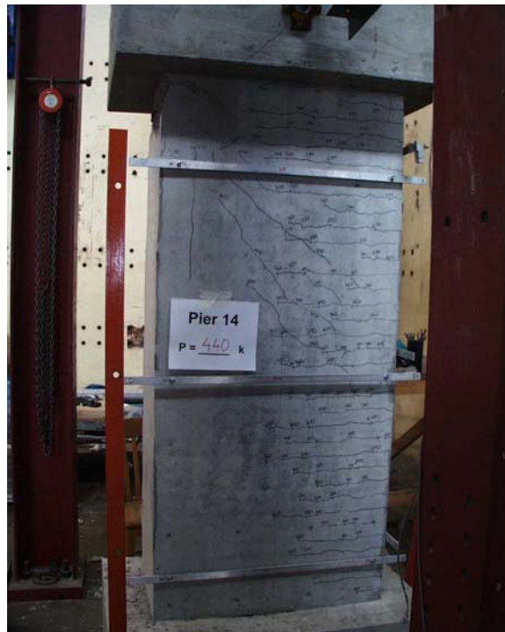
Figure 5.61 Specimen P14: Photo of West Wall at End of Test
