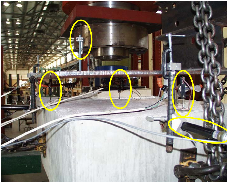
Figure 4.33 Linear Transducers (Black Instruments) Used to Measure Lateral Displacement of the Top End Block
