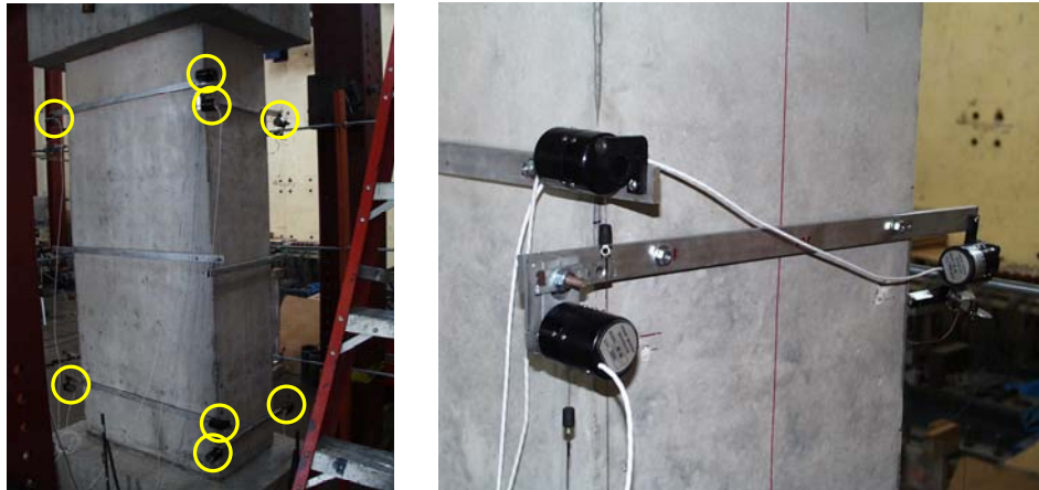
Figure 4.34 Instrumentation Used to Measure Curvature
