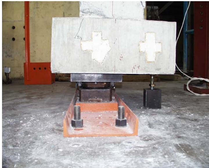
Figure 4.26 Spherical Bearing at Bottom End Block
