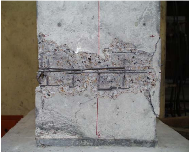
Figure 5.45 Specimen P12: Photo of North Wall at End of Test
