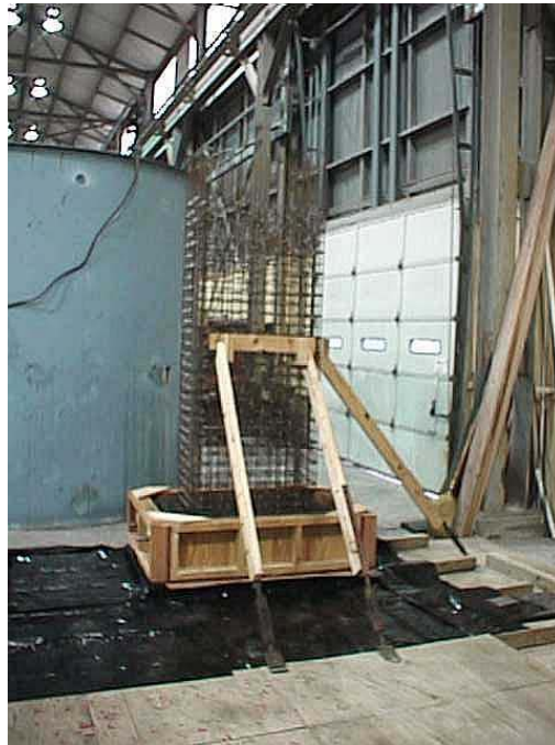
Figure 4.16 Bracing System Used to Align Vertically the Longitudinal Reinforcement
