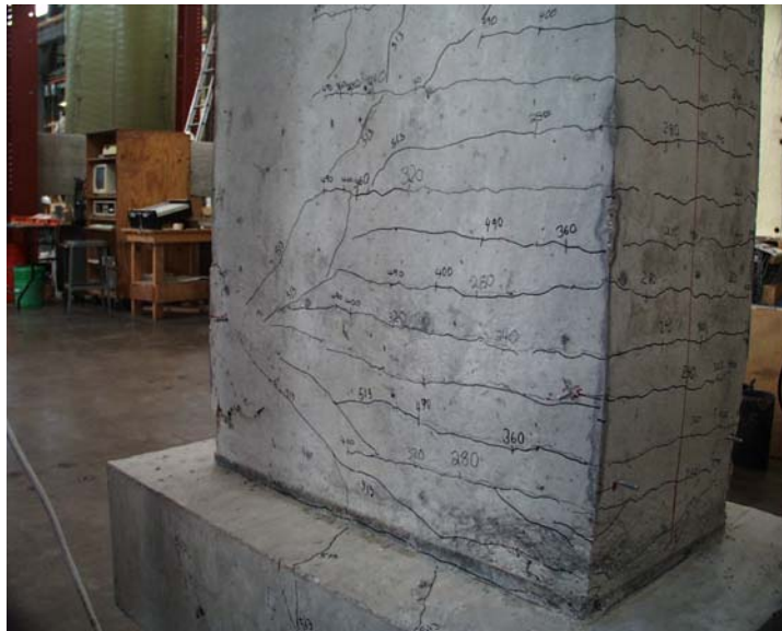
Figure 5.47 Specimen P12: Photo of West and South Walls at End of Test
